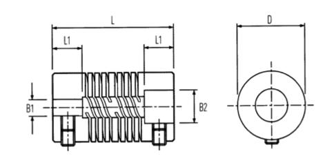
B1: Pre-drilled= 12.0B2: Pre-drilled= 25.00D= 63.5L= 150.0L1= 38.0Max angular displacement = 1.00Max B1 & B2= 38.00Max parallel displacement = 7
